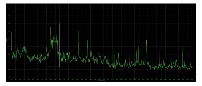
The display will adjust Frequency, span and reference level to the box you drew.
