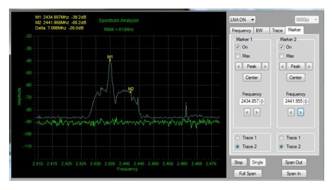
Markers are used to find amplitude at a frequency.
